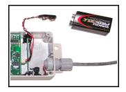
Replace battery with a 9-volt alkaline cell (Duracell MN1604B2 or equivalent).
