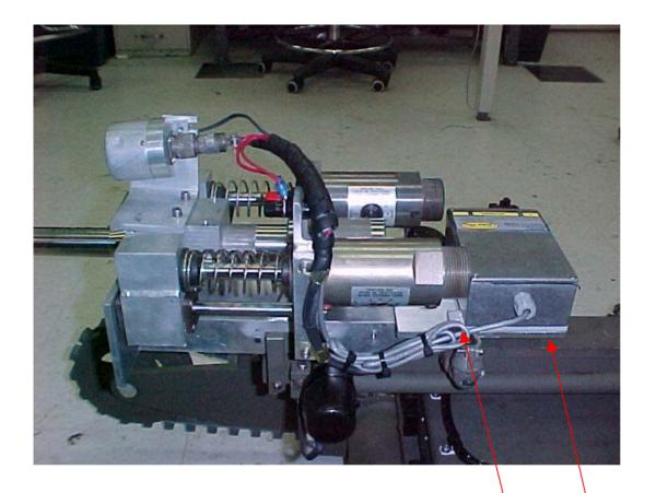
10-24x1/2 SST Socket Head Cap Screws and washers
